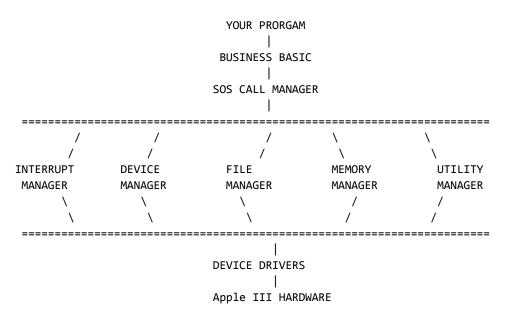
As you can see, each layer depends on the one below for services. Since the way the layers communicate is standardized on the Apple III, it is possible to make substantial changes to the hardware and even to some parts of the operating system without changing the way Business BASIC operates. This insures that your programs will continue to work, even if we make changes later. Designing operating systems this way takes longer, and makes them larger, but in the long run the benefits are enormous.
